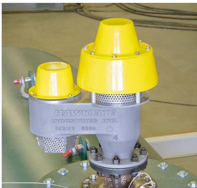
Series 6000 PVRV mounted on flow test apparatus, June 2017. Photo courtesy C-FER Technologies (1999) Inc.
