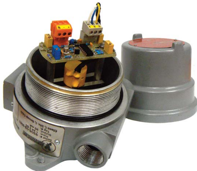
Above: Goshawk Transmitter with cover removed
