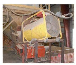
1 Million btu heater on chute that requires less than 2,500 btu to heat, which is 400 times more heat than required (400 times more cost).
