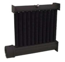
The *ExCaliber*™ vacuum sealed liquid-to-air heat exchanger core is constructed using rugged, copper-free, roll-formed aluminum fins and protected by a pressure relief device, automatic reset high limit, and a back-up manual reset high limit.
