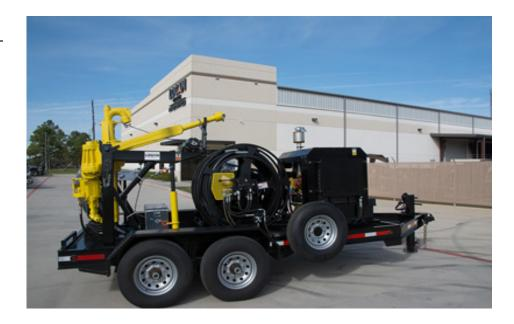
The newly engineered, hydraulic motor-driven, 85-Ton Power Swivel provides smooth, shock-free torque. It is rated to support tensile pipe loads of 85 tons at zero rpm and 45 tons of dynamic load at 100 rpm. The compact swivel head design weighs only 1,163 lbs. and fits into most drilling or workover masts.
