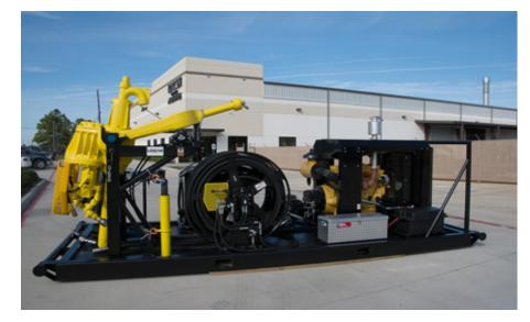
The newly engineered, hydraulic motor-driven, 120-Ton Power Swivel provides smooth, shock-free torque. It is rated to support tensile pipe loads of 120 tons at zero rpm and 65 tons of dynamic load at 100 rpm. The compact swivel head design weighs only 2,000 lbs. and fits into many drilling or workover masts.
