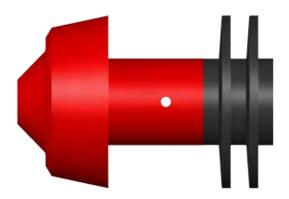
The unique design of our new dual durometer Hurricane FP pig has a front hollow mandrel with two port holes in the middle of the mandrel. This allows the inhibitor to travel to the front of the pig and then through the port holes. The inhibitor is then contained between the 86 durometer leading cup and two 62 durometer rear sealing discs allowing the pig to leave a film of inhibitor on the pipe wall.
