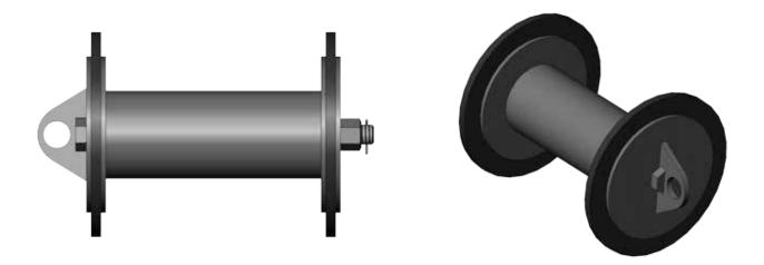
MD series, in sizes 14" and smaller, have a through bolt mandrel design, complete with a pull hook. Sealing discs experiencing wear after traveling one direction, can reverse direction without compromising their sealing characteristics. All discs are produced from Apache's special blend of wear resistant Reliathane.
