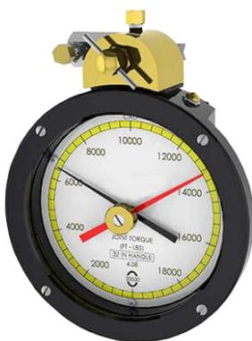
Indicates torque in foot pounds applied to each joint when using power tongs to run oilfield tubulars. These systems are available for all makes and models of power tongs and come with either compression or tension type load cells that provide an accurate check of make up torque for all oilfield tubulars. Dual scale variations are also available. Rugged, simple load cell designs guarantee extra long life and ease of maintenance.
