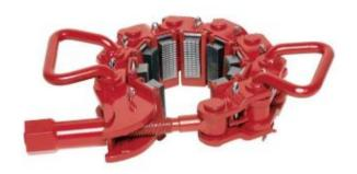
Safety clamps consist of tapered segments that wedge onto a tubular when the clamp is tightened. They help prevent slick or small upset tubulars from dropping downhole.
