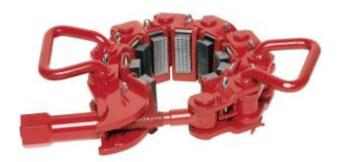
Type MP Safety Clamps are necessary tools for handling drill collars, flush joint pipes and small shoulder pipes. They could adjust pipes of different sizes by changing the quantity of chain links. They are designed and manufactured according to API Spec 7K
