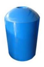
Guide Shoe is a simple and economical means to run casing in the well bore. All the internal components are fully PDC drillable. This design contains an internal taper on the bottom to ensure trouble-free entry of drilling tools back into the casing string after drill out and during drilling operation. Eccentric cement noses can be provided for applications where sloughing and highly deviated well bores are encountered. All Guide Shoes and internal components are fully PDC drillable.
